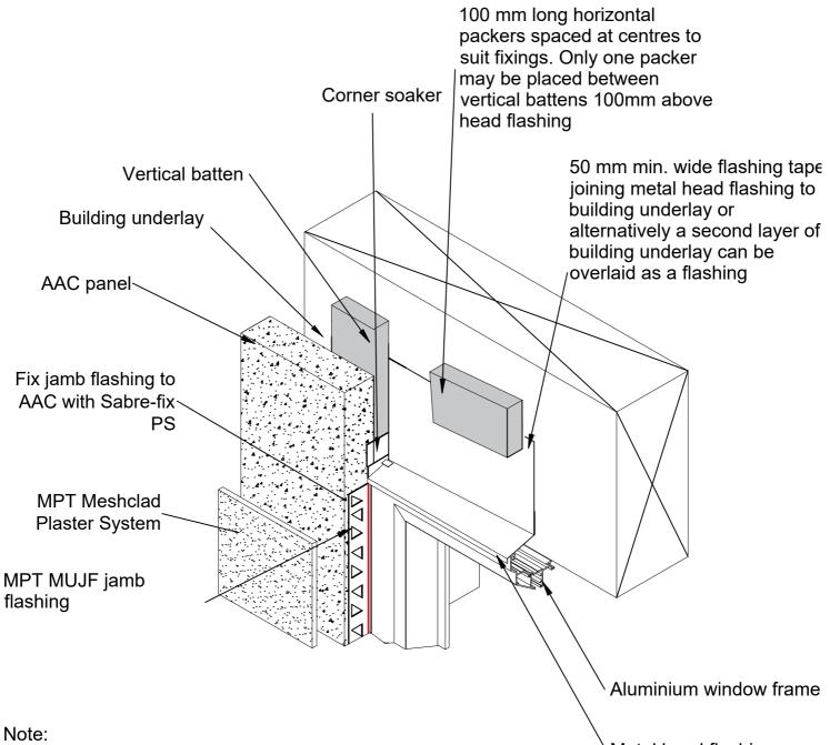
Diagonal mesh across all corners of windows and doors. Fiberglass mesh omitted for clarity Metal head flashing
