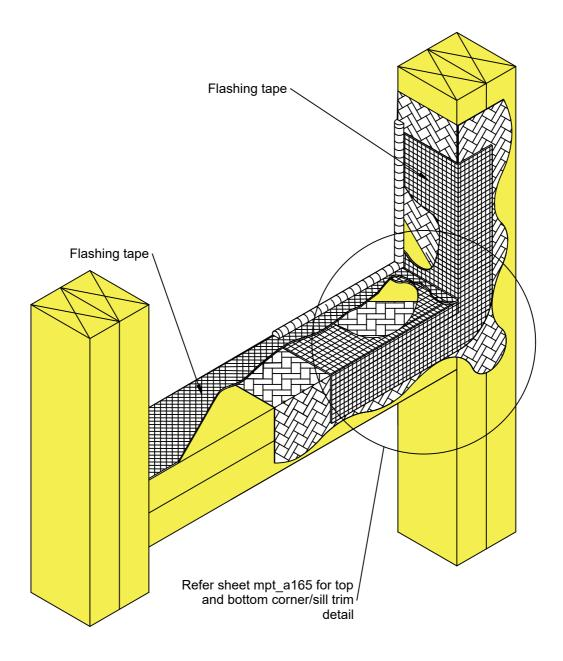
Note: A sloped sill trimmer is required when the glazing pocket of the window is located back past the line of the wall framing
