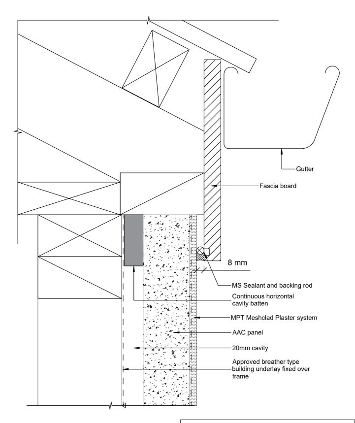
Note: Apply plaster before fascia board and gutter installed
