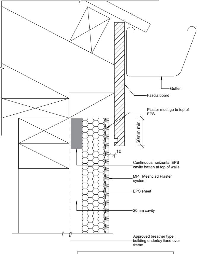
Note: Fascia board installed after cladding is plastered
